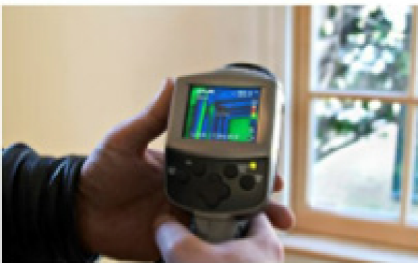
Photo of Infrared Camera in Use: Many Home Energy Raters use infrared cameras to pinpoint areas where heat and cold can escape from a home so they can be sealed and properly insulated by the builder.
